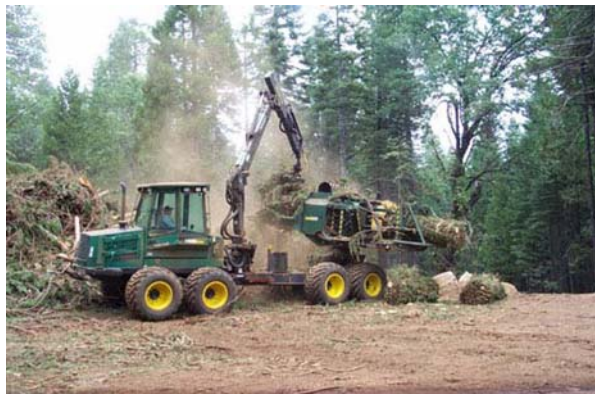
Fig. 1 Photograph of JD 1490 Slash Bundler on a study site showing use of boom grapppler to feed biomass into the compression jaw, compression of biomass into a bundle, and exit of bundle from compression system after binding with twine
